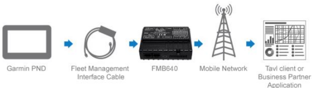
Figure 82 FMB640 +Garmin operational scheme
